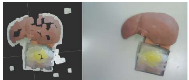
Fig. 4 Qualitative 3D reconstruction of a cholecystectomy phantom.
