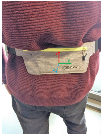
Fig. 1: Smartphone belt, smartphone position and reference axes
