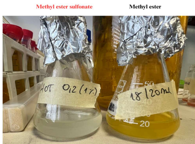
Figure 8. The transparent product indicates the methyl ester sulfonate (left flask), while the methyl ester before sulfonation appears yellow (right flask).
