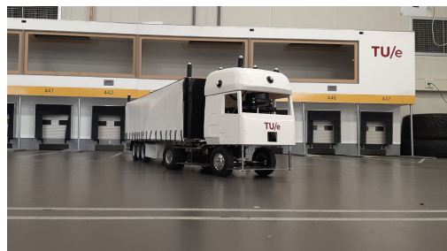
(b) Truck and semi-trailer model with a reduction ratio of 1:13.3 in Automotive lab
