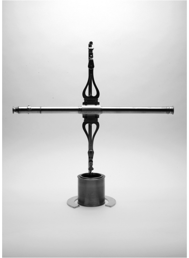
Fig. 2. Jan Pauw, Automatic water level instrument , 1796, Leiden, Museum Boerhaave. This machine was invented by Christian Huygens in 1679.
