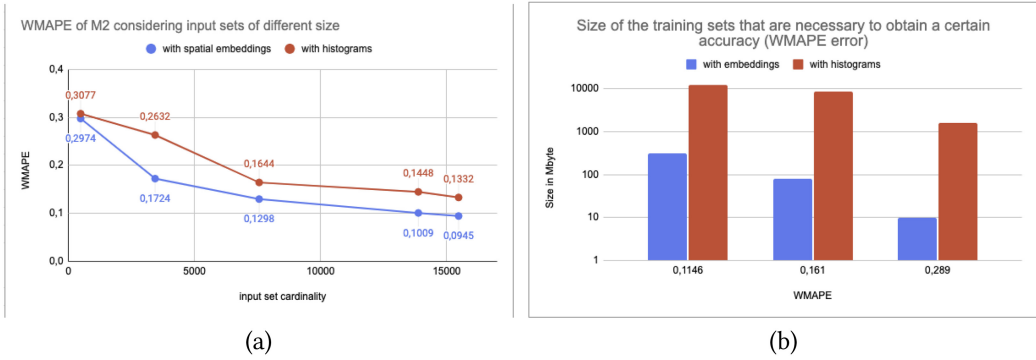
Fig. 7. Comparison among M2 models trained with spatial embeddings or directly with histograms. In (a) the WMAPE error for the two cases is shown as the cardinality of the training set is increased, while (b) compares the size in MByte of the input sets needed for the two cases for obtaining the same WMAPE values.
