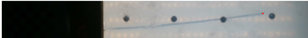
Figure 4.9: An example frame with the needle tip estimation represented as a red dot
