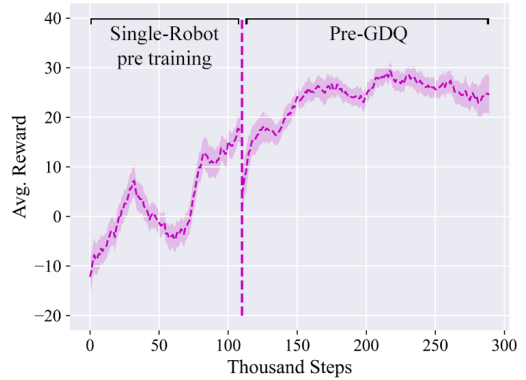
Fig. 6. Avg. reward for the single-agent pre training (left) and Pre-GDQ (right) initialized with a single-robot policy that reached \approx 20 avg. reward. Pre-GDQ reaches \approx 30 avg. reward in around 210000 steps.
