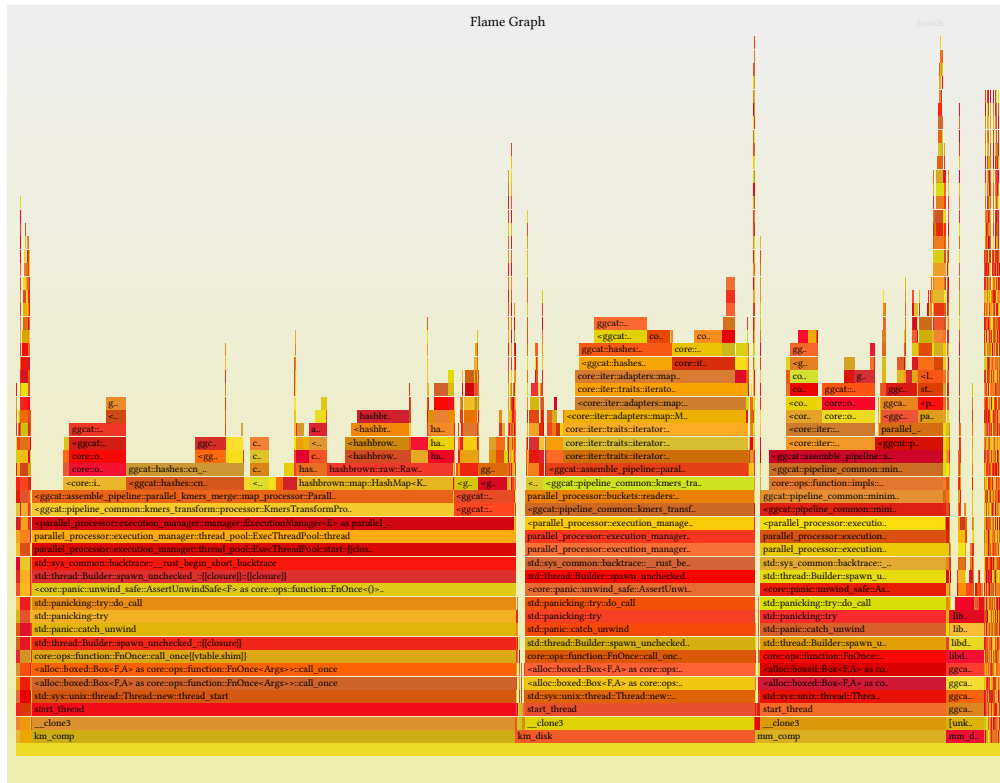
Figure 36: An example of a flamegraph generated using cargo-flamegraph while profiling GGCAT. The x-axis size represents the proportional time spent in each function, while the stacked bars represent nested function calls.
