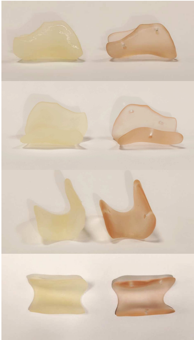
Figure 46 Different views of the grids. On the left, the PEGDA-printed grid; on the right, the resin-printed grid
