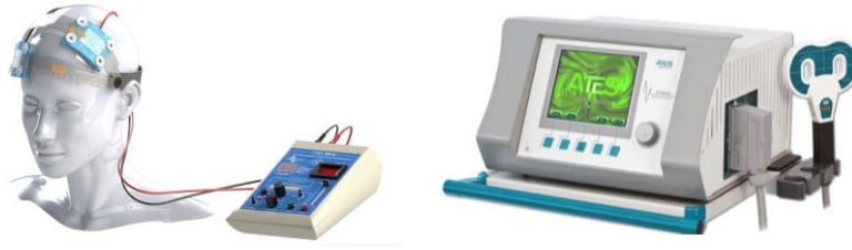
Figure 1. tDCS and TMS apparatus. On the left, the tDCS apparatus. It comprehends a device for the current supply and two electrodes put on the scalp. On the right, the TMS equipment. It is composed by a capacitor for the generation of a powerful and rapid-discharging electrical current, which flows into a figure-of-eight coil placed on the scalp. Images taken by Wikipedia.
