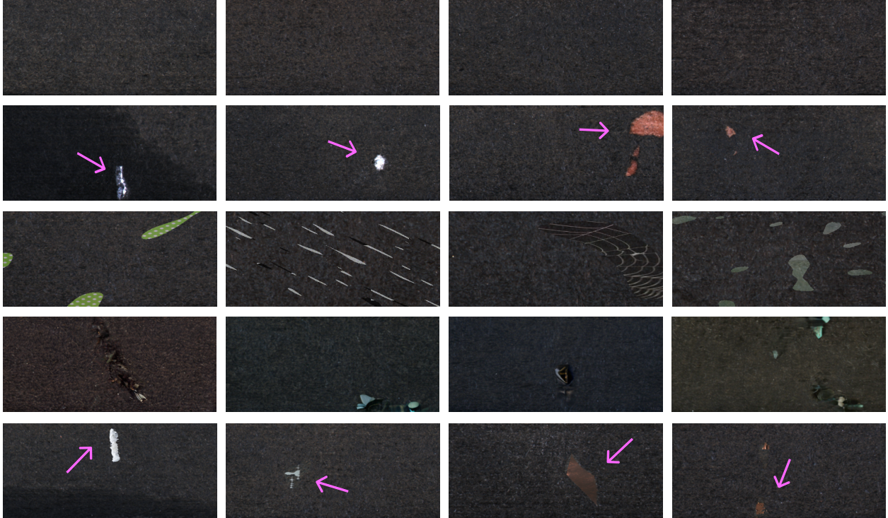
Figure 5.2: First row displays some negative samples from the KSDD2 dataset. Instead, the second row shows some images of positive samples from the same dataset. In the third row, we show the MemSeg-generated defect samples. The fourth row shows In&Out generated defect samples. Lastly, the final row showcases images generated with DIAG. Notably, the defect images that DIAG generated are more realistic and in-distribution.
