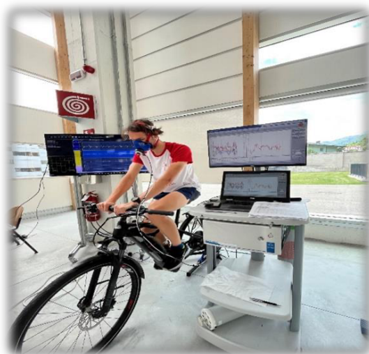
Fig. 5.2 Set-up of data collection during phase two of the study using the metabolic cart and surface electromyography.
