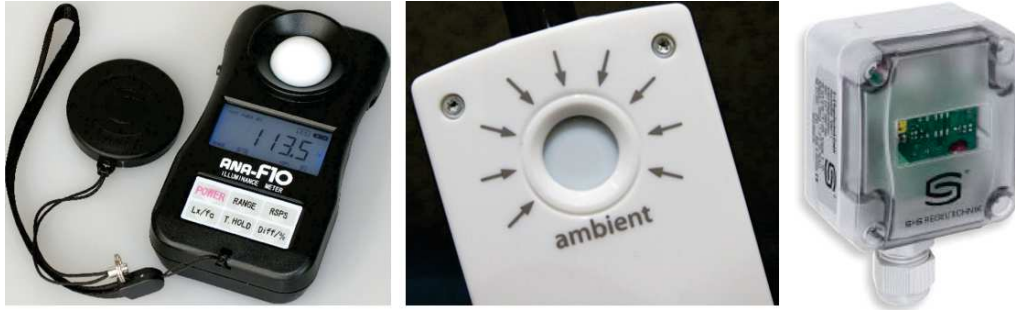
FIGURE 2.2: Various commercial illuminance meters (luxmeters), that we also used in this thesis in order to obtain ground truth light measurements.
