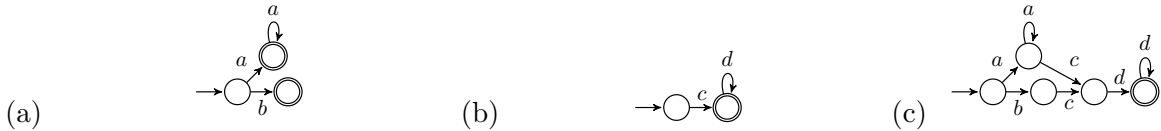
Figure 10: (a) A , \mathcal{L}(A) = \{a^n \mid n \in \mathbb{N}\} \cup \{b\} (b) A' , \mathcal{L}(A') = \{cd^n \mid n \in \mathbb{N}\} (c) A'' = \text{CC}^\sharp(A, A')
