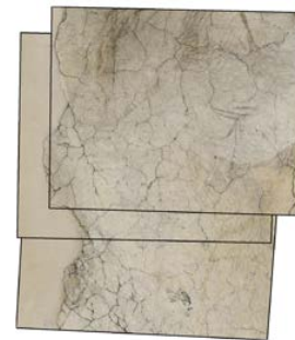
Figure 12: From left to right: mosaic of three emissivity frames; light corrected emissivity mosaic following [28]; visible orthophoto.
