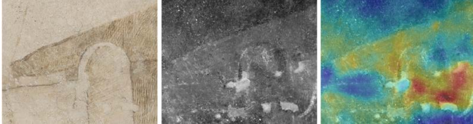
Figure 10: Example of dual-mode imaging for diagnostics in a fresco detail: visible (left); TQR measurement (center); alpha fusion image between TQR and thermogram after the lamps switch-off (right).
