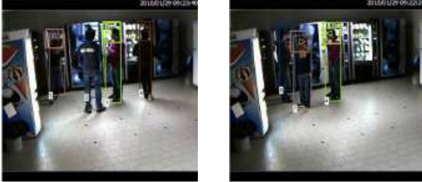
Fig. 5.8. Examples of tracking and head orientation classification results. The largest box represents the tracking estimation, the smaller box the area where the head is positioned, and the triangle depicts the estimated head orientation.
