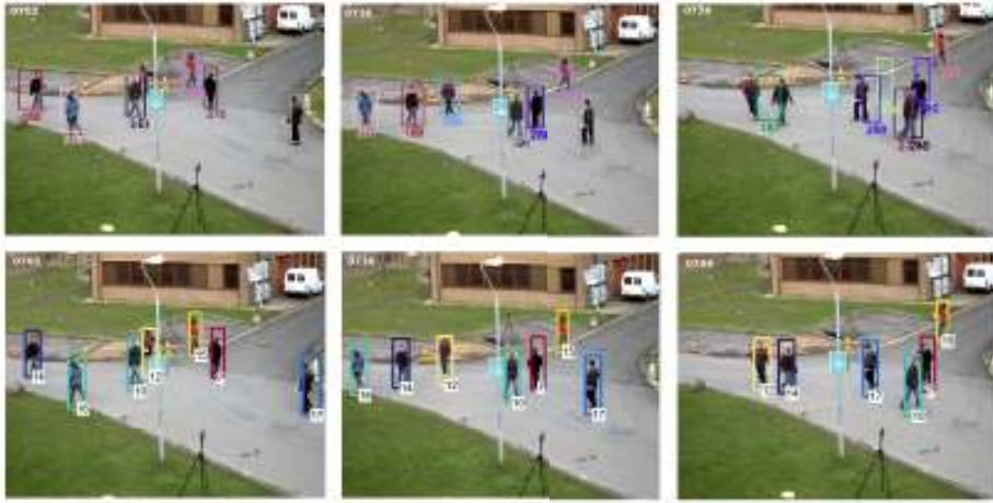
Fig. 2.7. Tracking results for frames 702, 716, and 736 of task S2, video L1, View001: first row shows MHKF and second row show HJS filter.
