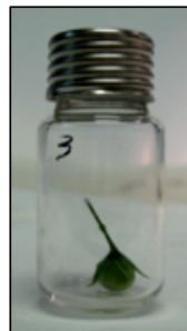
Fig. 20: Example of ethylene analysis: a berry of S. neorickii in a chromatography vial (11 ml).
