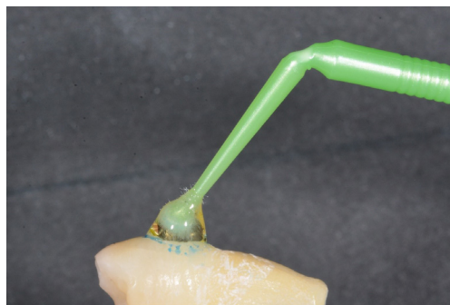
Figure 5. Application of Scotchbond Multi-Purpose© Adhesive with a microbrush for 1 minute on the marked area
