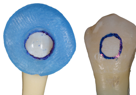
Figure 1. Blue wax mold used to mark a repeatable circular area on every dental element, as shown on the right
