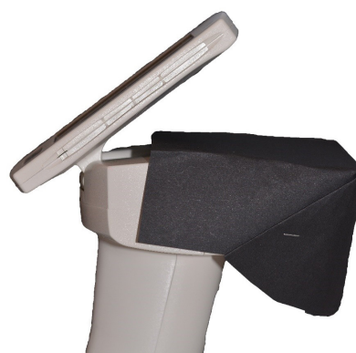
Figure 9. Black cardboard applied around the spectrophotometer sensor
