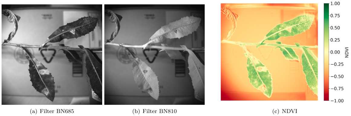
Fig. 15. Images acquired in laboratory with the MSX multispectral camera. (a) BN685 filter (675–692 nm) shows higher reflectance where the infection has reached the leaves, (b) while the BN810 filter (798–820 nm) shows the necrotic areas (lower reflectance) where there is no more chlorophyll. (c) NDVI is the Normalized Difference Vegetation Index.
