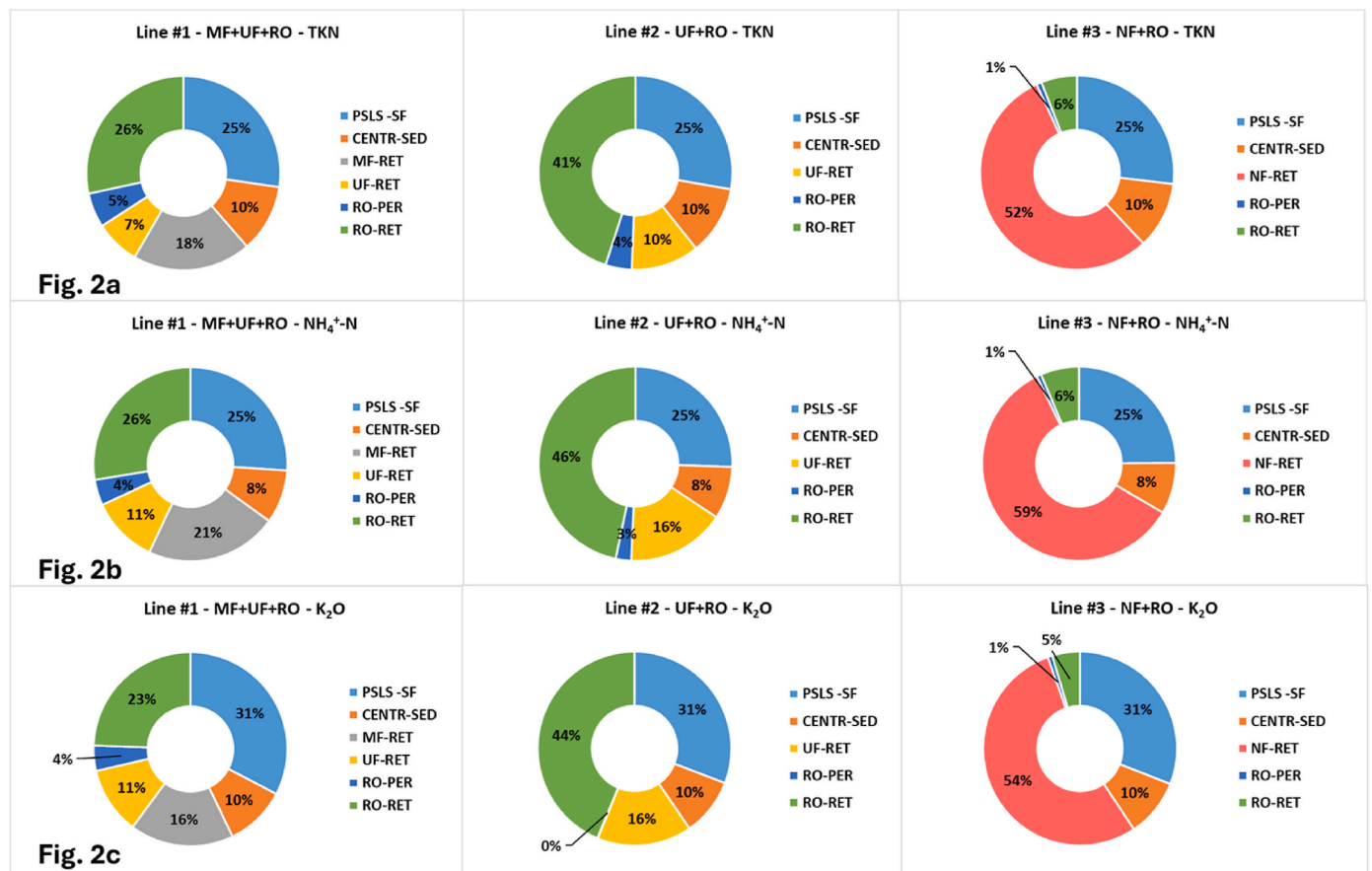
Fig. 2. Distribution of Total Kjeldahl Nitrogen (Fig. 2a), ammonium (Fig. 2b) and Potassium as K 2 O (Fig. 2c).
