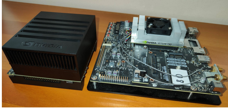
Fig. 4.7: The embedded platforms used for testing. The Nvidia Jetson Xavier (left) and Nvidia Jetson TX2 (right).
