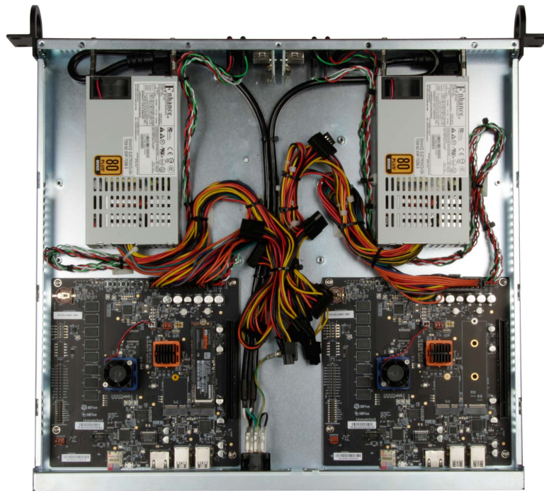
Fig. 2.5: The Monte Cimone Server Blade hosts two SiFive Freedom U740 SoCs and has a form factor of 4.44 cm (1 RackUnit) in height, 42.50 cm in width, and 40 cm in depth. Each RISC-V board has dimensions of 170 mm by 170 mm.
