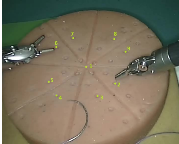
Fig. 9.4: Right camera endoscope image extracted from trial 22 showing the rotated positioning of the phantom. Numbered points indicate ordered fiducials used for spatial calibration
