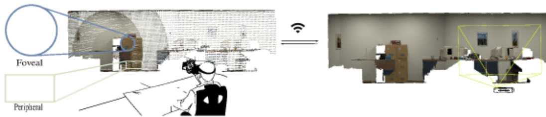
Figure 3.1: Foveated rendering in VR of a real-time 3D reconstructed remote scene. The user’s gaze itself is used to foveate the remote point-cloud. The scene is rendered with dense points in the fovea region and progressively sparse rendering in the peripheral regions.
