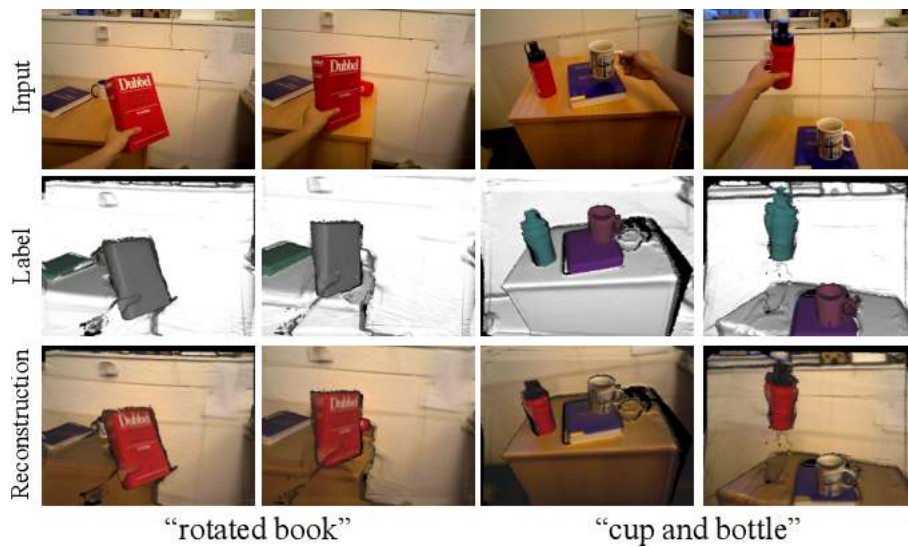
Figure 2.17: Qualitative demonstration of the work MID-Fusion [176] input RGB (top row), semantic class prediction (middle row) and geometry reconstruction result (bottom row).
