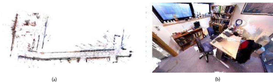
Figure 2.15: (a) Sparse reconstruction of a map using feature-based approaches [101] and (b) a dense reconstruction of an office [170].
