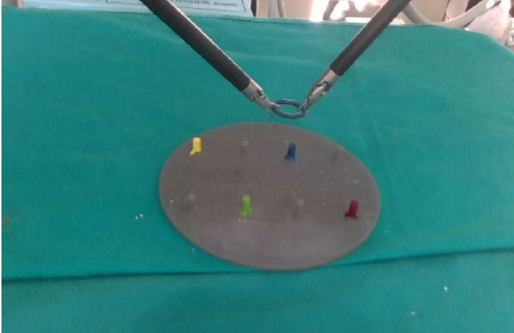
Fig. 3.6: Dual arm manipulation experiment. The two arms carries a ring while performing circular trajectories through the workspace.
