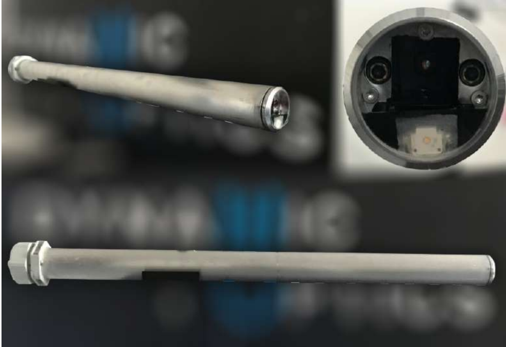
Fig. 2.5: The first prototype of the depth stereo endoscope
