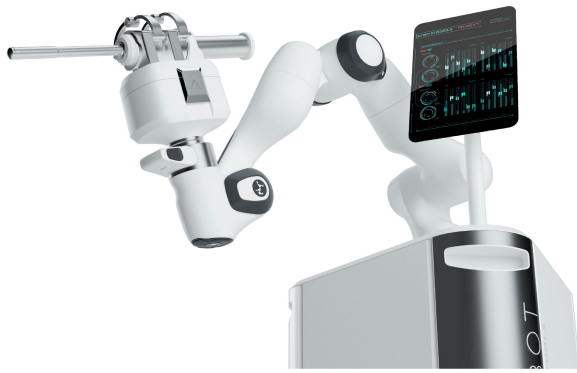
Fig. 1. Artist rendering of the prostate biopsy positioning head (PROST) as a component of a larger robotic system, that may be used also for other procedures. For the experiments described in this paper, the robotic head was mounted on a wheeled cart.
