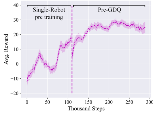
FIGURE 8.7: Average reward for the single-agent pre training (left) and Pre-GDQ (right) initialized with a single-robot policy that reached \approx 20 avg. reward. Pre-GDQ reaches \approx 30 avg. reward in around 210000 steps.
