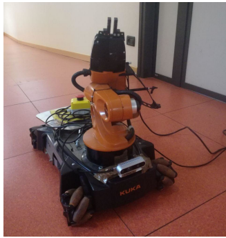
Figure 3.24: The YouBot with the Realsense D435 camera on its front.
