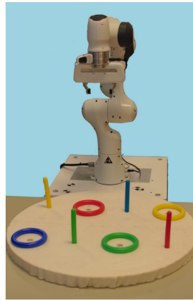
Figure 7.13: Robotic setup for the Peg & Ring task with the Panda industrial manipulator.
