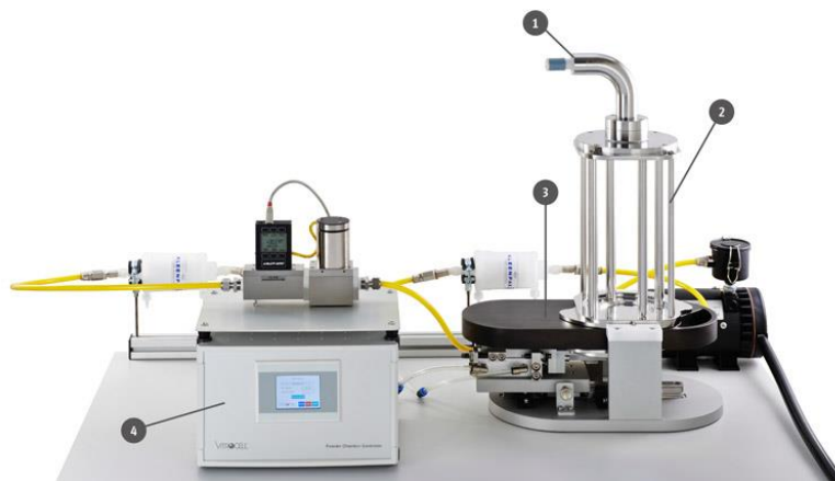
Figure 17. Vibrocell® exposure system for dry powder can be applied from all commercially available inhalers or via direct dosing (Taken from Vibrocell® Systems website).
