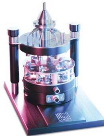
Figure 15 CULTEX® RFS module (Taken from Cultex® website)
