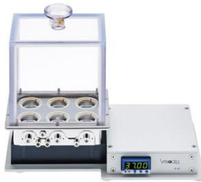
Figure 16. Vibrocell® exposure system for liquid aerosols with single droplet sedimentation (Taken from Vibrocell® Systems website).
