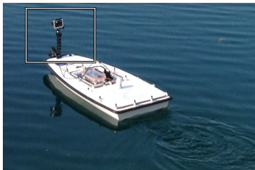
Fig. 3.5: IntCatch 2020 project uses Platypus Lutra boats, about 1m long and 0.5m wide.
