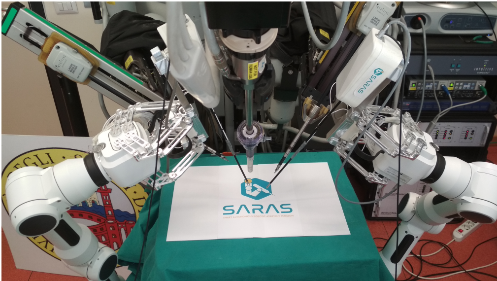
Fig. 4.9: SARAS experimental setup: the two white arms in the foreground are the novel laparoscopy arms being developed for the SARAS project; the endoscope (in the middle) and the two robotics arms in the background are the daVinci ® surgical system arms connected to the DVRK [32] platform
