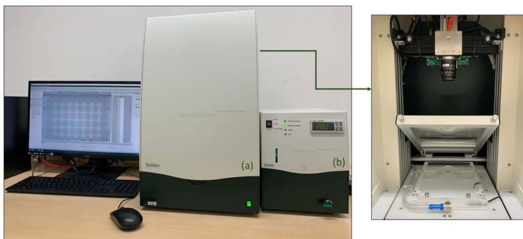
Figure 8: DanioVision apparatus: in the left the observation chamber (a), then represented open with the infra-red camera; in (b) the temperature control unit.
