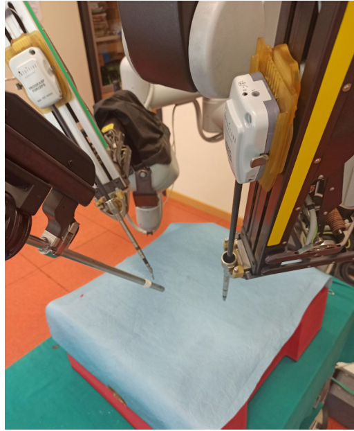
FIGURE 2.1: The patient side of the dVRK, with the PSMs (lateral) and the ECM (center).
